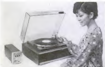
A SEEMING IMPOSSIBILITY —playing four channels from a single record groove—is accomplished by this Japanese Victor decoder to be marketed soon. It will work with any high-frequency phono pickup
